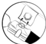
If the buoy is not positioned correctly in the pocket, proper release cannot be guaranteed!
