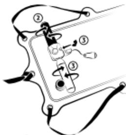
2 - Unscrew the used water activator and replace it with a new one.
